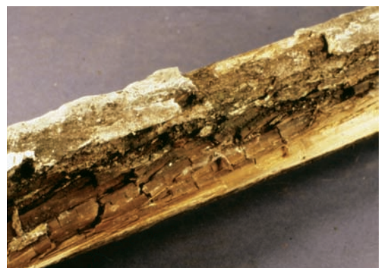
ABOVE (TOP): Fig. 1. Bacterial slime from within a pipeline. COURTESY JOHN GILLATT, THOR UK LTD.
